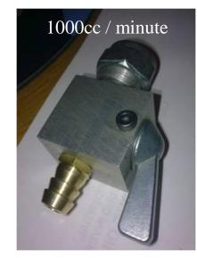
This tap body was made to suit the internals from a Hi-Level 8mm inline tap. The aluminium threaded boss,
