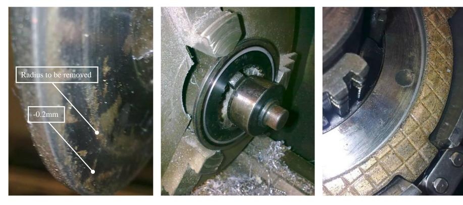
Clutch drum face showing 0.2mm step worn where first friction plate has been driving.
