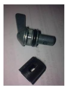
Here are the internals from the Hi Level tap. Rather than dump the main body from the tap, if you clean off the paint and saw it up into pellets, you can use these as the filler to connect the aluminium threaded boss to the billet body, by using a propane torch and the same technique as you would for Lumiweld, HTS2000 or similar.
